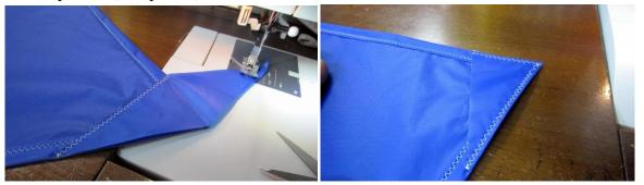
4) Place 1 sail back side down on work surface. Place 16" aluminum ring holder with ring added at top bridle point placing it ½" into this seam, see photo. Repeat for lower bridle point with 2" aluminum ring holder with ring in place. Align 2<sup>nd</sup> half of sail on top of first with good side down. Sew both sides together 3/8" from edge on ¾" sew line from drawing 4
