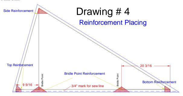
1) Mount and sew all reinforcements where indicated other that the side reinforcements on the back side of sail. Drawing 4.
